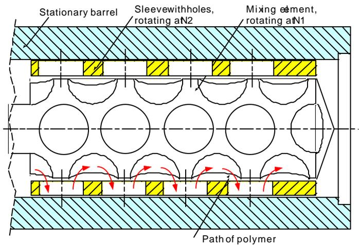
Figure 4, Representation of the Twente Mixing Ring
