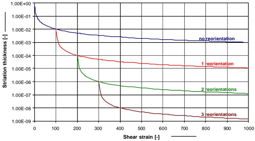
Figure 2, Striation thickness versus shear strain with reorientation
