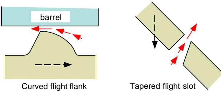
Figure 2, Two methods of creating elongational flow in the CRD mixer
