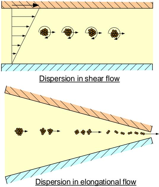
Figure 1, dispersion in shear and elongational flow
