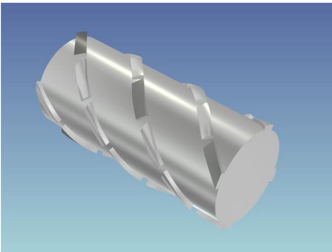
Figure 3, Three dimensional rendering of a CRD5 mixer
